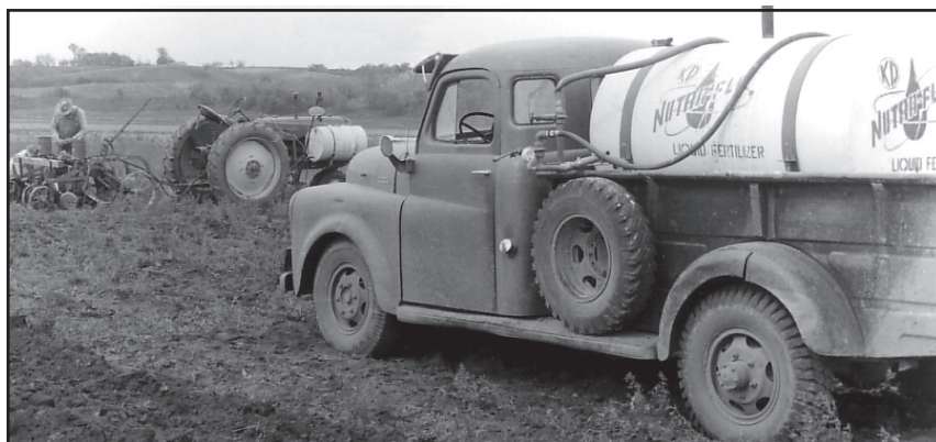
Here’s a picture of Nutra-Flo’s first nurse truck delivering starter fertilizer to a grower at planting time. Notice the 50-gallon barrel saddle tanks on the tractor.
